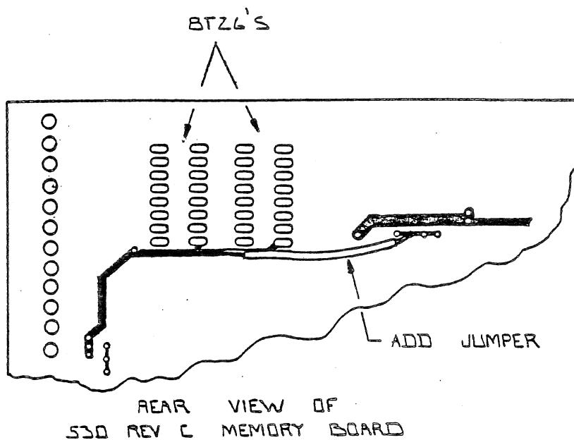
We have received reports of trouble with the 530 dynamic memory boards operating spuratically. We are currently looking at the trouble. The change shown above decreases ground noise between the 8T26's and the memory array. The jumper should be 18 gauge or heavier wire. The jumper should go from the tape that runs between pin 8 of the two 8T26's to the ground pad near the memory as shown above.
