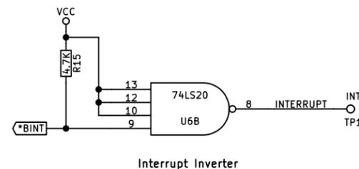
If desired, jumper output to one of the 8085 interrupt inputs
