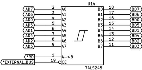
Data Bus Buffer and Control Logic
